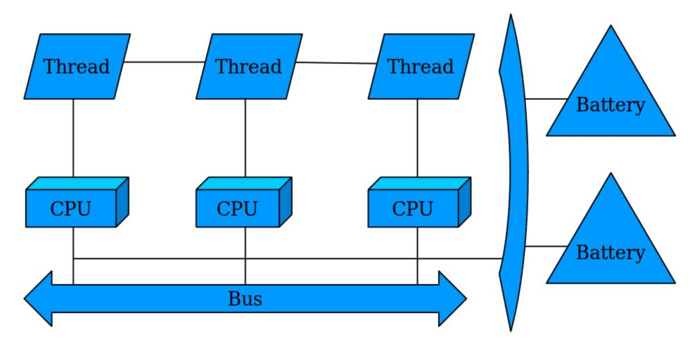
A battery has a matrix of cells, and each cell has a current level of charge. A battery scheduler determines parallel and sequential connections between groups of cells in order to satisfy voltage and current output requirements.
